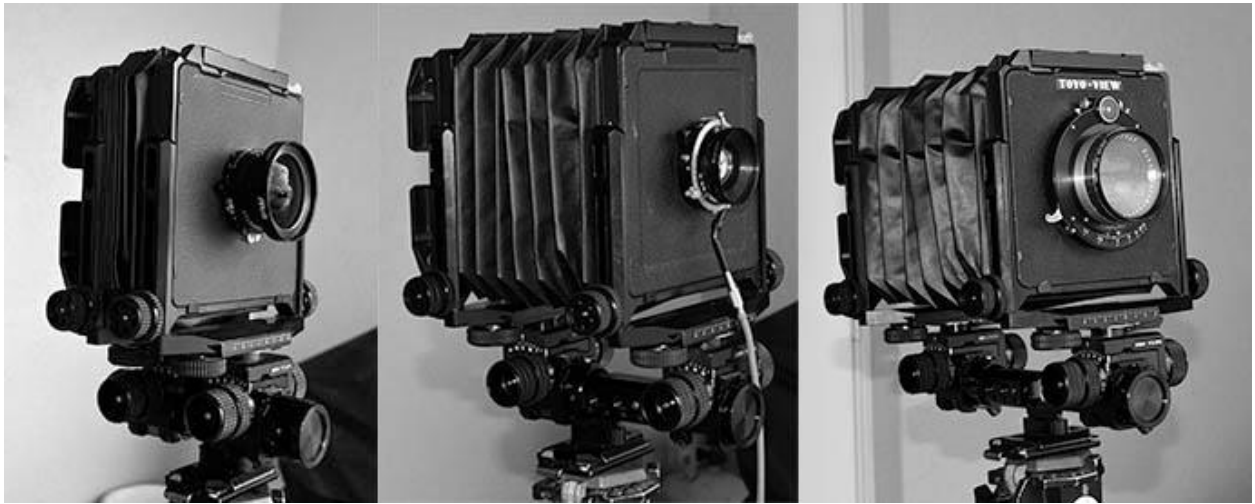
Photo 3.3 - Photographs showing the amount of bellows extension needed on lenses of different focal lengths. The photo to the left is a 75mm lens. The lens in the middle is a normal 150mm lens. The photo on the right is a 240mm telephoto lens.
