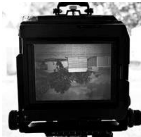
Photo 3.2 - The image will appear upside down on the ground glass. Use a loupe to make fine focus adjustments on the camera.
