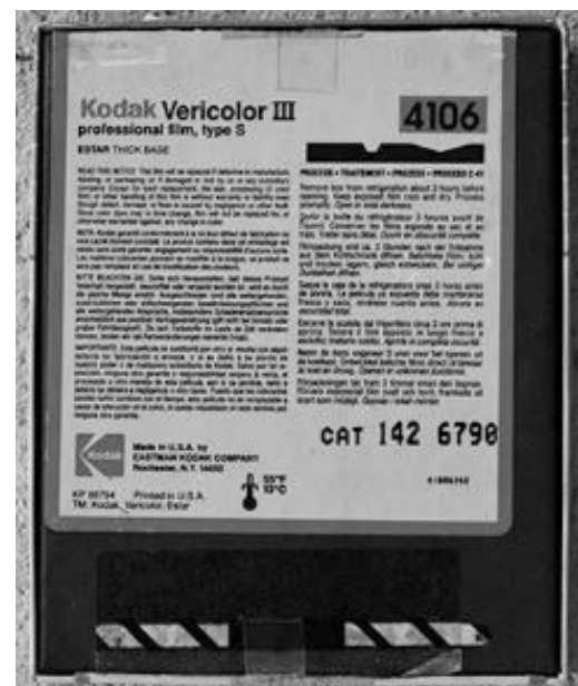
Photo 2.1 – On the back of film boxes and envelopes is a drawing that shows the identifying notches are cut in the film. You see it just below the numbers "4106" on this box of film. Each type of film has its own specific markings.
