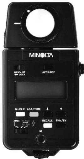
Photo 7.2 - Incident light meters measure the light falling on a subject instead of light reflected from a subject.
