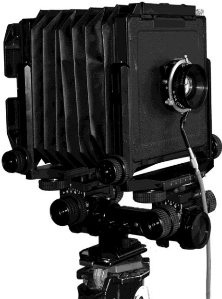
Photo 6.1 - Always start by straightening and leveling your camera. If you get confused while making movements on your camera, return everything to normal and start over.
