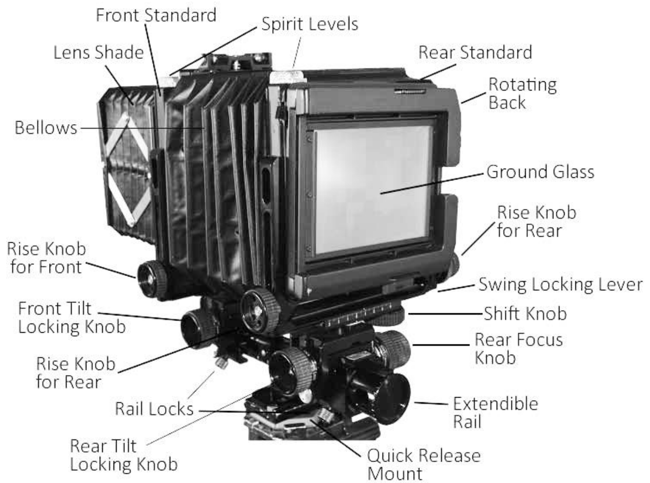
Photo 4.2 – Typical parts and features on the back of a view camera.
